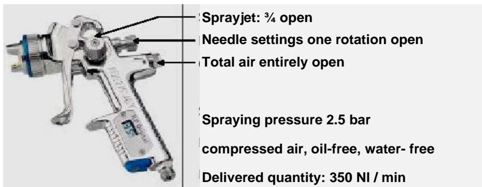
**Attention:** Wear breathing equipment when spraying because of the creation of aerosols. Ensure sufficient aspiration.
